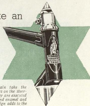
*Nameplates again take the place of transfers on the steering heads. They are executed in chromium and enamel and their smart design adds to the appearance of the models. Note also the fish-tailed lugs.*
