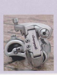
REAR DERAILLEUR: the operating principles of the Stratos rear derailleur are those derived from the higher range groups with which it is completely compatible. The new rollers designed for use with the new chain have also been adopted in the Stratos rear derailleur for further enhanced shifting. All the components of the mechanism are articulated on self-lubricating bushings which ensure longer life.
