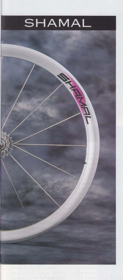
EXTREME WHEEL LIGHTNESS. THANKS TO THE SPECIAL RIM PROFILE AND THE USE OF ONLY 16 SPOKES, THE WEIGHT IS LOWER THAN THAT OF A TRADITIONAL WHEEL. THIS LIGHTNESS, FURTHER REDUCED BY USING CASSETTE HUBS WITH AN ALUMINIUM FREEWHEEL, ALLOWS THE INNOVATIVE FEATURES OF THE SHAMAL WHEEL TO BE EXPLOITED ON ANY TERRAIN, WHILE CLIMBING.
