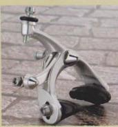
BRAKES: The new Athena brakes are the caliper type and use the innovative MONOPLANER system of interfacing the levers themselves. This particular design makes it possible to work the two blockholders on the same plane and ensures braking which is perfectly balanced between the blocks with the elimination of all vibrations. The block-holder levers are in hotpressed aluminium alloy and are anodized after polishing, a characteristic of Campagnolo products.
