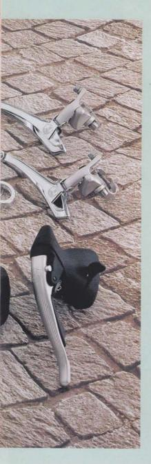
BRAKES: Veloce brakes are the essential expression of functionality and reliability. The CAD designed block-holder levers are in hot-pressed light alloy which ensures maximum strength, an essential feature of a safety product such as brakes. The blocks are the result of long studies carried out by Campagnolo to guarantee safe braking in all conditions of use.
