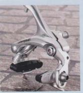
BRAKES: devised with the innovative double fulcrum system, Chorus brakes are in hot-pressed aluminium alloy, the only solution capable of guaranteeing maximum resistance to breaking. All the articulations are made with self-lubricating bearings and bushings. The double possibility of adjusting the return spring setting and balancing the brake itself with the rim means that the use of the brake can be personalized depending on the bike and user.
