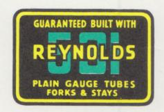
The Top Tube, Seat Tube and Down Tube of a frame which bears this decal are REYNOLDS 531 BUTTED tubing. Fork blades and stays are of lesser quality.
