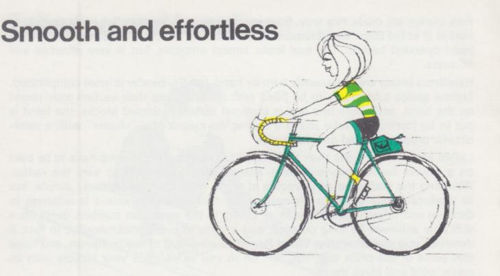
Modern road surfaces are generally good—but even so, if our front forks were rigid we would have a very uncomfortable ride, and use up so much energy absorbing the vibration in our arms that mileages would tumble and times would stretch alarmingly. So the front fork blades are curved to a carefully planned "rake" to provide resilience and so smooth out some of the road-roughness.
