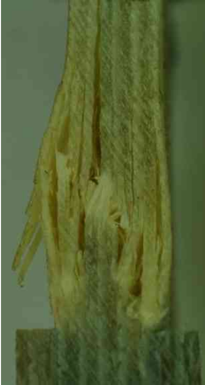
Figure 28: Buckling of plies and secondary delamination
