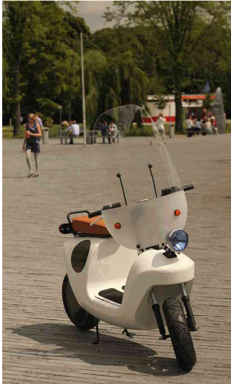
Figure 59: This 'bioscooter', an electrically driven scooter made of biocomposite materials, was developed in a joint venture with Hogeschool Inholland.
