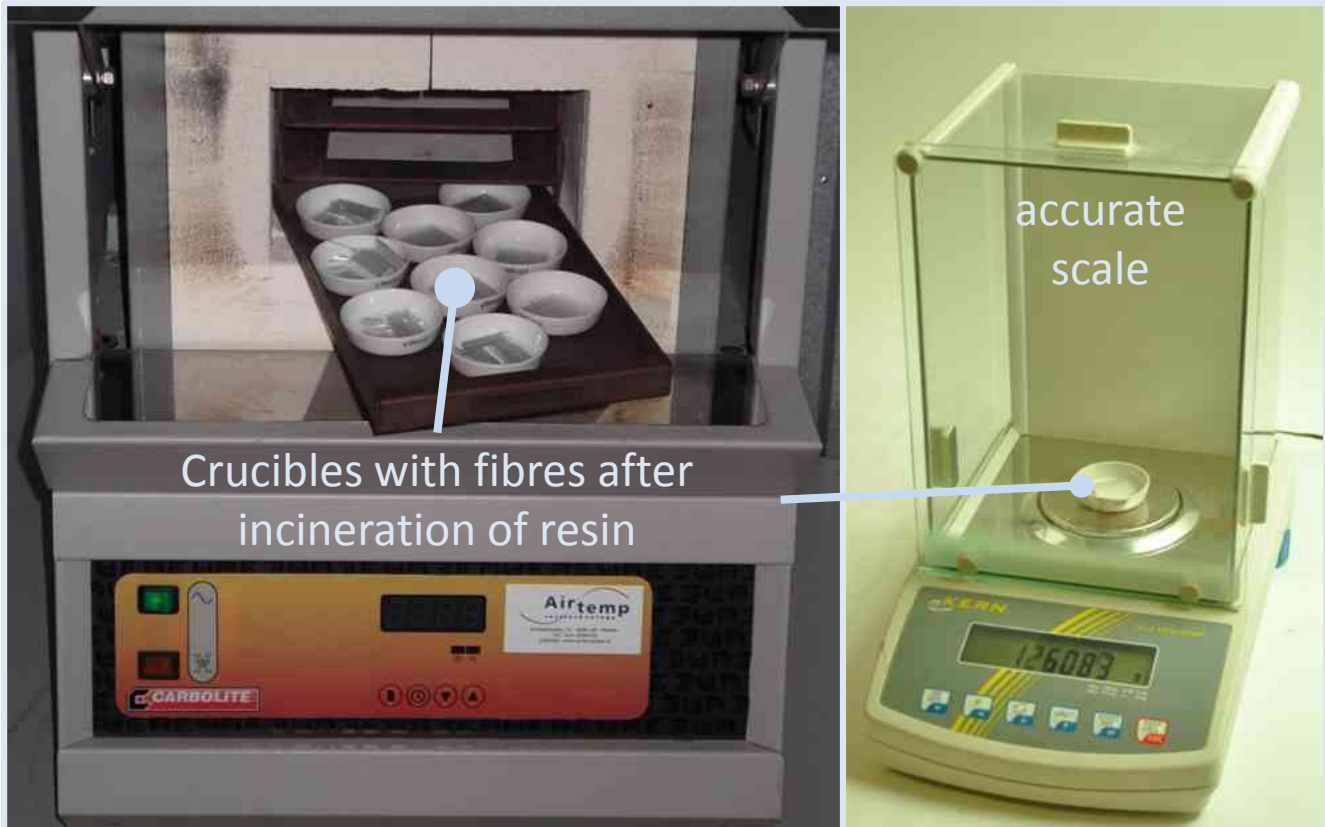
Figure 68: Accessories for performing fibre volume content measurement (source: WMC)
