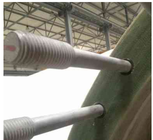
Figure 53: Joints in the plane of the laminate by means of an insert at the blade division location [2] and at a blade root of a wind turbine rotor blade (source: TRES4/EOZEN)
