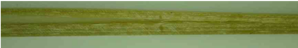
Figure 27: Delamination (source WMC)
