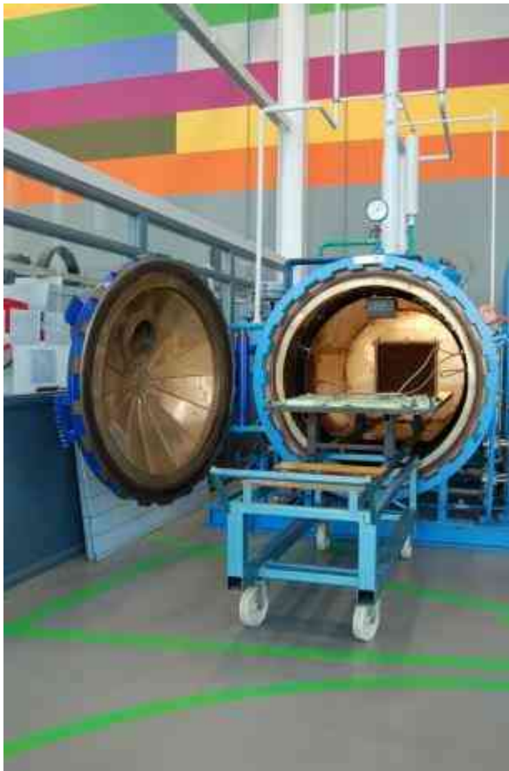
Figure 25: Autoclave at the composites lab, INHolland, Delft
