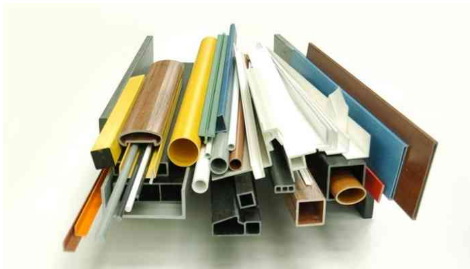
Figure 22: Pultrusion is pre-eminently suitable for the production of various profiles [2, 3]
