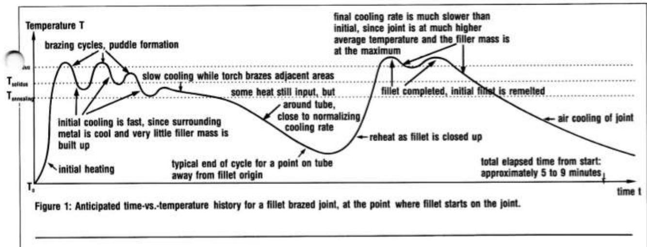
Figure 1: Anticipated time-vs.-temperature history for a fillet brazed joint, at the point where fillet starts on the joint.
