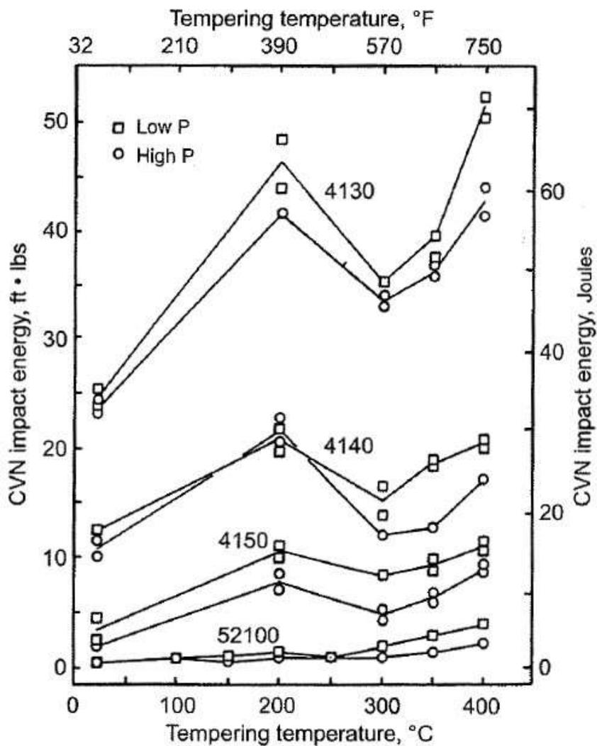
Brittle failure is the most dangerous kind of failure. Attempting to temper with a torch at ~200C (light yellow oxides) where there is a peak in toughness, little drop in UTS and a sizable increase in yield strength may be tempting, but there is a risk of overheating with poor torch control and it is unlikely you can achieve the appropriate soak times required.
