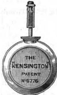
spring draws it half-way down the side of the nozzle, the end of this portion of the can being free for the egress of the oil. By simply pulling up and drawing into position, the cap drops into its place at once, and is pressed firmly upon the top of the nozzle by the spring, and thus prevents the oil oozing out.
