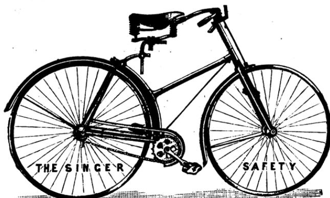
5in. centres. Elliptical handle-grips, 30in. bent back hollow, detachable, adjustable bars. Singer's frame of  $1\frac{1}{4}$ in. 15 W.G. weldless steel tube.  $\Gamma$  seat pillar with side bolt adjustment. Townsend's combination spring and saddle. Circular step. Pull-up lever hinged plunger spoon brake on front wheel. Mud-guards over both wheels and chain. Spanner and oilcan. Weight 46lbs.
