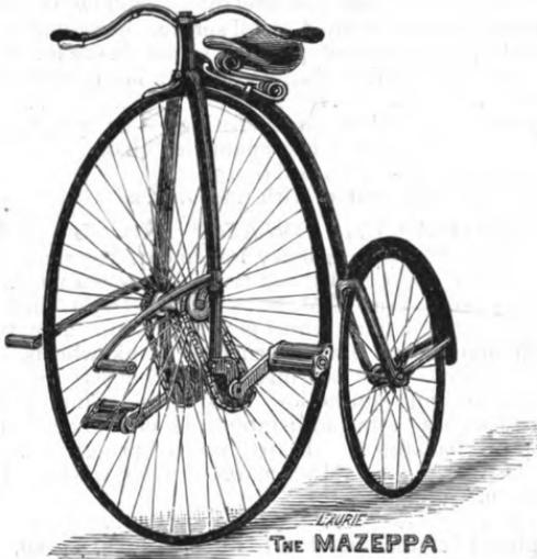
like ordinary bicycle. Forks 2in. behind bearings. Hollow front and semi hollow back forks. Stanley head, 4in. centres. Pear-shaped horn handles, 28in cowhorn bars. Weldless steel backbone. Arab cradle spring. L.D. suspension saddle. Circular step. D.L.S. brake. Leg-guard. Valise, spanners, oilcan, lamp, and bell. Weight 40lbs.
