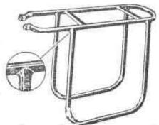
"CONTINENTAL". Light triangular support from platform to mudguard eyebolt, on drop-out. No clips to chip enamel, top support from brake pivot bolt, will take Release fittings, finished in Silver 10/6 FRONT. Similar, bolts over pivot bolt and hub spindle ... 12/6
