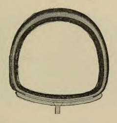
pneumatic, but in place of a thick body of rubber the Indestructible has five thicknesses of twilled linen duck wrapped in such a way as to bring the laps over each other at the tread, where the puncture is liable to occur, and making punctures practically impossible.
