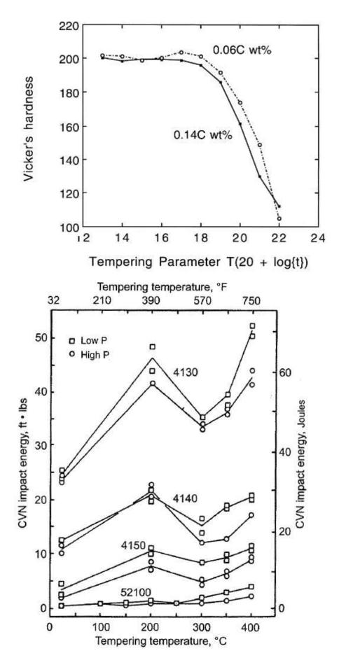
Brittle failure is the most dangerous kind of failure. Attempting to temper with a torch at ~200C (light yellow oxides) where there is a peak in toughness, little drop in UTS and a sizable increase in yield strength may be tempting, but there is a risk of overheating with poor torch control and it is unlikely you can achieve the appropriate soak times required.
