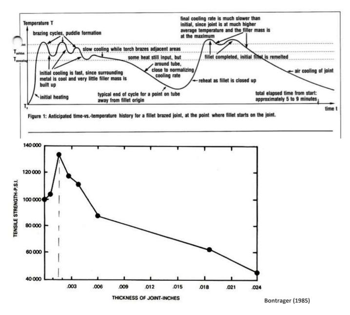
The effect of reducing stress risers is also largely not necessary. Welded frames hold up fine with very small fillets. Main tubes are loaded primarily in compression and tension, not bending (Allen, 1982). Large fillets do have some advantages, the most significant probably being aesthetics. Large fillets likely do help distribute stresses, even if it is unnecessary. In the case of poor miters, large fillets probably add strength to the joint by acting as a non-penetrating bronze weld.
