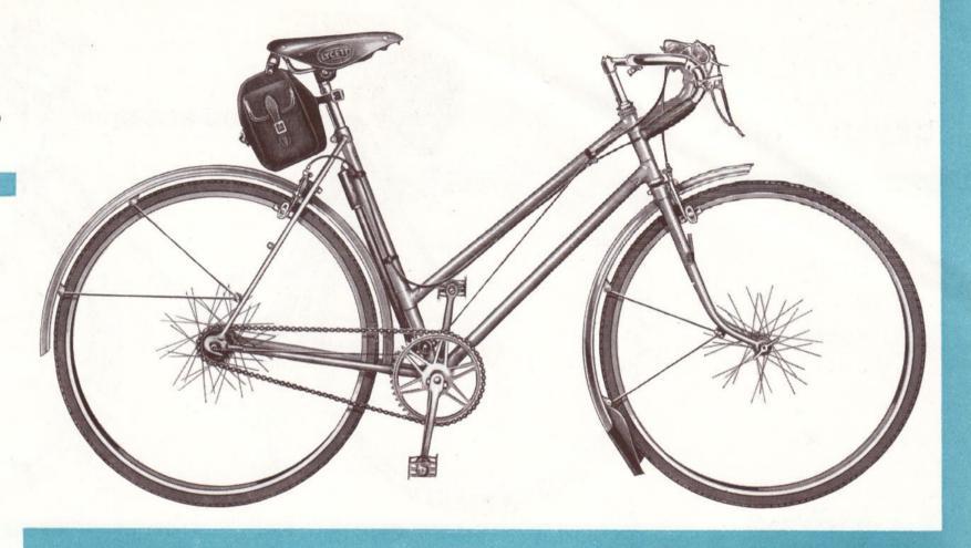
FRAME: Sizes 20", 21", 22" and 23", brazed up back stays and brazed on fittings, cut-away and fish-tail lugs.
