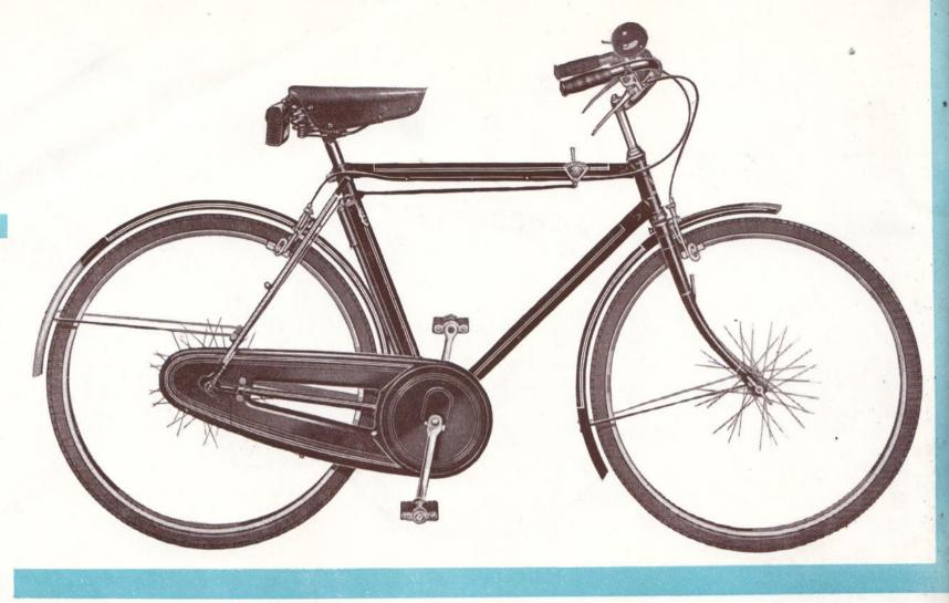
**FRAME**: Built in sizes 20", 21", 22" & 23" brazed up. WHEELS:  $26" \times 1\frac{3}{8}$ " Endrick pattern.
