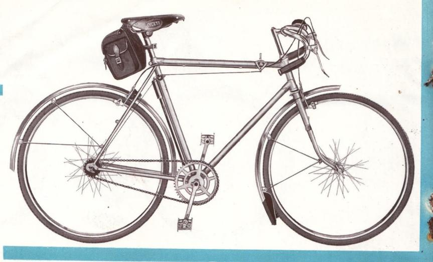
FRAME: Sizes 20". 21", 22" and 23", brazed up back stays and brazed on fittings, cut-away and fish-tail lugs.
