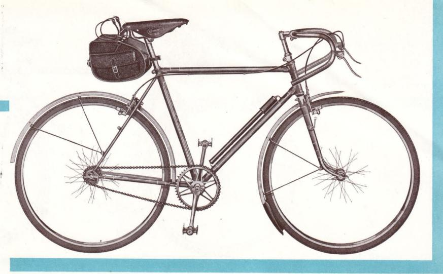
FRAME: Sizes 21", 22" and 23" in 531 Tubing. Brazed up back stays, brazed on mudguard and reflector eyes, cable clips and pump pegs. Angles: 73° Head, 71° Seat.
