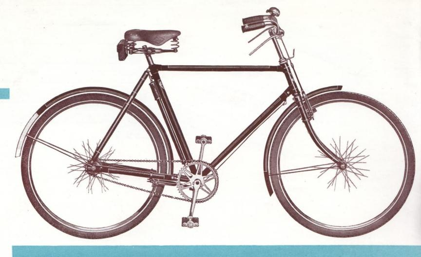
**FRAME**: Built in sizes 20", 22", 24" with  $10\frac{1}{2}$ " ground clearance.
