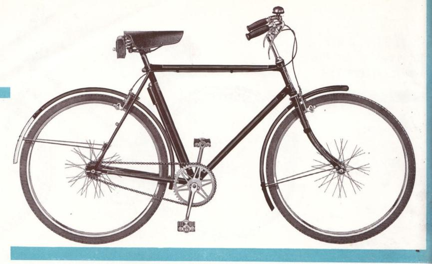
**FRAME**: Built in sizes 20", 21", 22" & 23" brazed up. WHEELS:  $26" \times 1\frac{3}{8}$ " Endrick pattern with rustless spokes.
