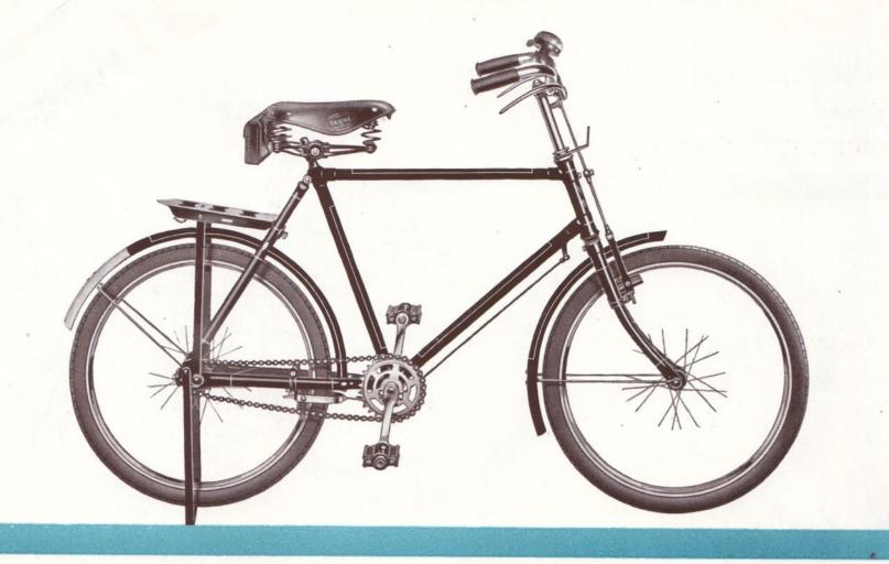
FRAME: Sturdily built brazed up frame in sizes 16" and 18" with 18" and 20" rims.
