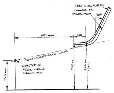
FIGURE 4: Semi-Recumbent Pedaling Position
