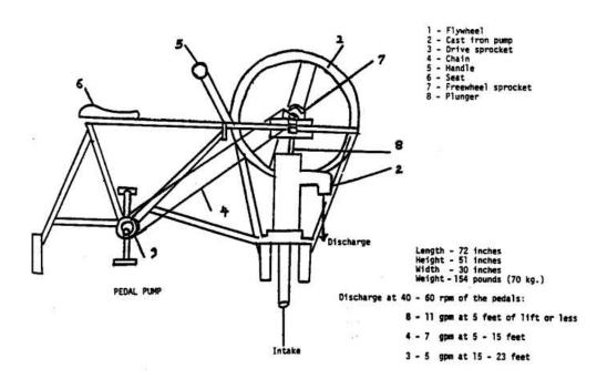
FIGURE 6: Pedal Powered Irrigation Pump
