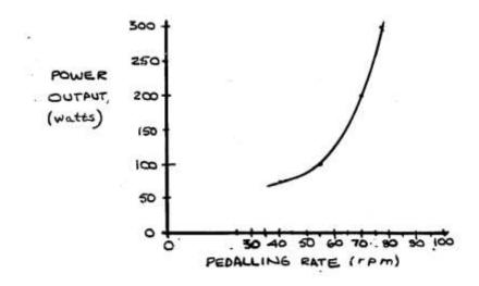
FIGURE 2: How Optimum Pedaling Rate Varies with Desired Power Output
