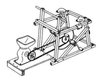
FIGURE 5: Two-person Dynapod with Chaindrive Operating a Grain Mill. Chainwheel is shown on left-hand side for illustration only.
