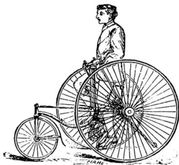
Fig. 21.—The Leicester Safety, 1881-2 (first bicycle front-steering tricycle).
