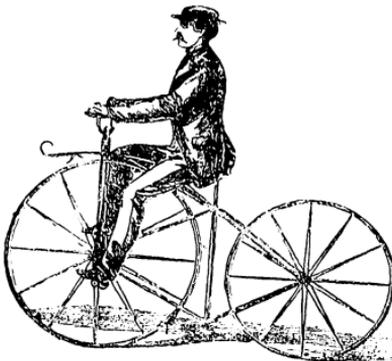
Fig. 10.—The Phantom double-steering bicycle.
