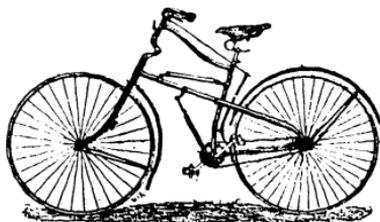
Fig. 37.—A spring frame Safety (the Whippet).
