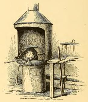
Fig. 4.-Forge Arranged for Tempering.
