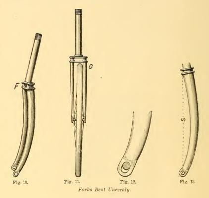
the other, F in Fig. 10. After bringing both forks forward so they are apparently straight, and lining them up in the usual way so the axle is parallel with the fork crown, the wheel is put in, and it is noticed that the wheel does not center in the fork, but is one sided, as at G in Fig. 11. This has been very poorly repaired by filing the hole up higher in the lower part
