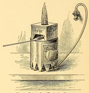
Fig. 5 .- Unique Case Hardening Furnace.
