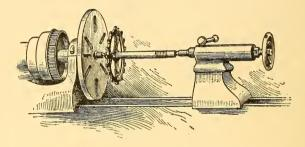
Fig. 20.—Truing a Sprocket Wheel,
