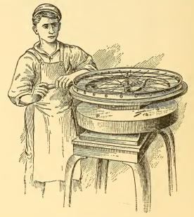
Fig. 1.—Assembling a Wheel.
