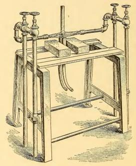
Fig. 5.-A Simple Brazing Furnace.
