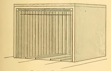
Fig. 10.-Steam Heated Enameling Oven.
