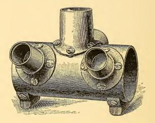
Fig. 9.—Fitting Parts for Brazing.
