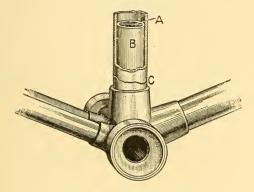
Fig. 12.-Mending a Broken Tube.
