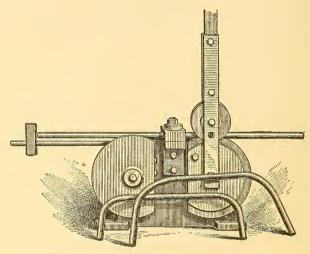
Fig. 4.—Machine for Bending Handle Bars.
