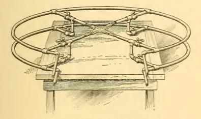
Fig. 4.-Four-Flame Brazing Furnace.
