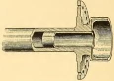
Fig. 23.-Mending a Broken Hub.
