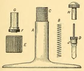
Fig 4.—Repairing the Valve Proper.
