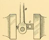
Fig. 5.--Vise Used for Removing Crank Key.
