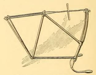
Fig. 3.—Pulling a Bent Fork Into Position.
