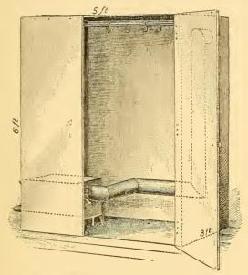
Fig. 8 .- Enameling Oven Heated with Coal.
