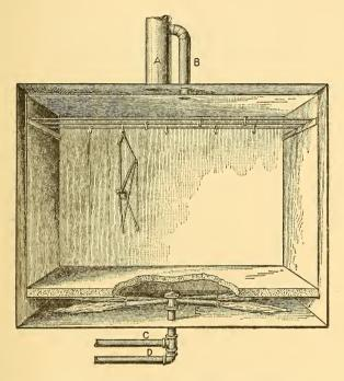
Fig. 6.—Enameling Oven Heated from Outside.
