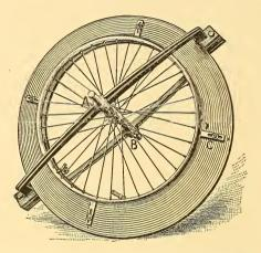
Fig. 2.—Frame for Stringing up a Wheel.
