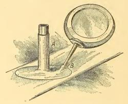
Fig. 1.—Repairing Inner Tube Valve Stem.
