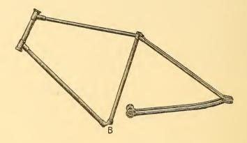
Fig. 2.—Crank Shaft Bracket Broken.
