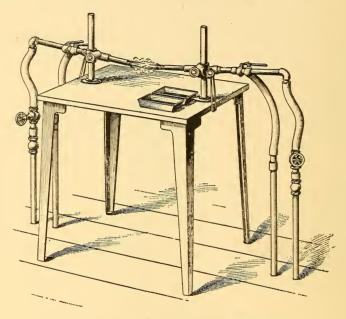
Fig. 3.—Brazing Furnace Without Fire Bricks.
