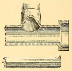
Fig. 1.—Removing a Ball Bearing Case.
