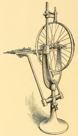
Fig. 7.—Jack for Holding a Wheel for Truing.
