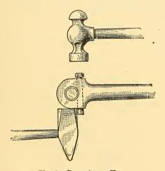
Fig. 2.—Removing a Key.
