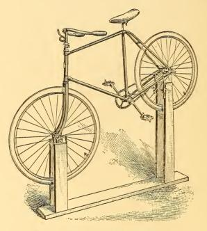
Fig. 1.—Supporting Bicycle at Bearings.
