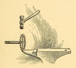
Fig. 19.—Removing a Screwed on Sprocket.
