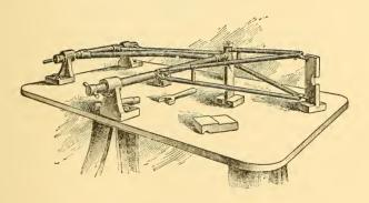
Fig. 20.—Table for Testing a Frame.
