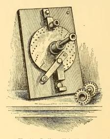
Fig. 15.-Drilling Hub Flanges.
