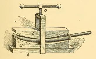
Fig. 4.-Bending Forks.
