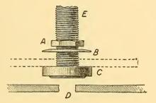
Fig. 2.—Repairing a Single Tube Valve.
