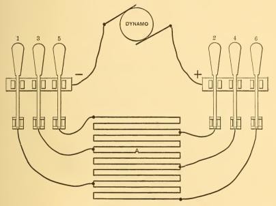
Fig. 9.-Electrically Heated Enameling Oven.
