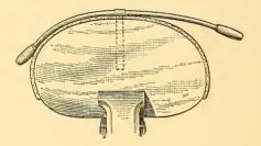
Fig. 1.-Form for Bending a Handle Bar.
