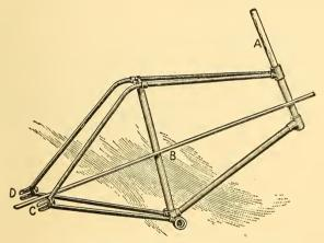
Fig. 17.—Truing a Frame with a Straight Edge.
