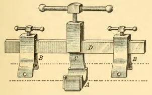
Fig. 14.—Device for Straightening Tubing.
