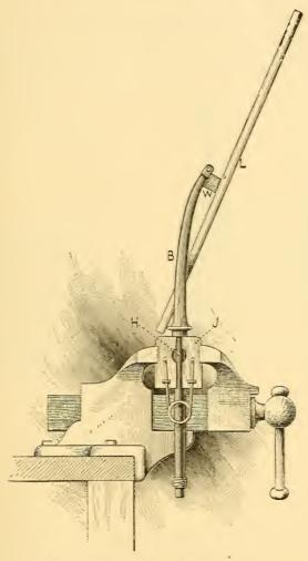
Fig. 9 .- Holding Fork in Vise for Bending.
