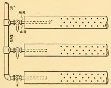
Fig. 3.—Plan of Multiple Bunsen Burner in Fig 2.
