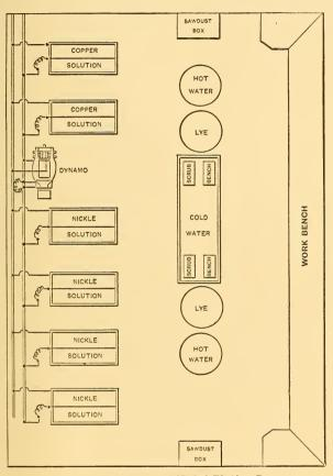
Fig. 1.—Arrangement of Nickel Plating Room.
