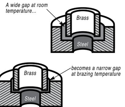
Of course, the same principle holds in reverse. If the outer part is brass and the inner part steel, you can start with virtually a light force fit at room temperature. By the time you reach brazing temperature, the more rapid expansion of the brass creates a suitable clearance.
