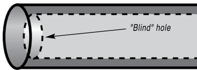
For years the cylinders were machined out of solid bar stock, with considerable labor required to drill and bore the blind holes. Finally, someone suggested that the cylinder was actually *two parts*—a tube and a plug.
