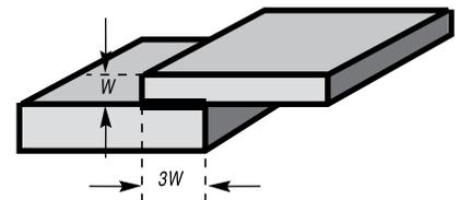
A longer lap may waste brazing filler metal and use more base metal material than is really needed, without a corresponding increase in joint strength. And a shorter lap will lower the strength of the joint. For most applications, you're on safe ground with the "rule of three."
