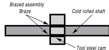
key, no set screw. Minimum material, minimum labor—and a strong, permanent, vibration-proof bond.
