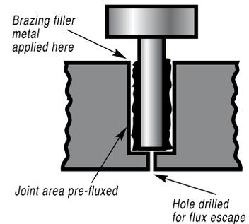
To maximize *corrosion-resistance* of a joint, select a brazing filler metal containing such elements as silver, gold or palladium, which are inherently corrosion-resistant. Keep joint clearances close and use a minimum amount of filler metal, so that the finished joint will expose only a fine line of brazing filler metal to the atmosphere.
