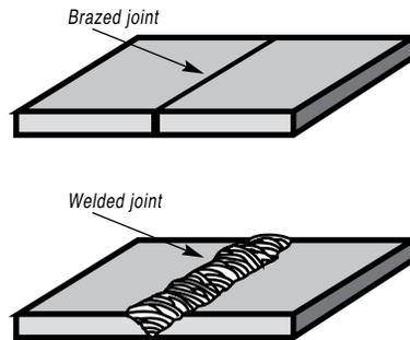
This characteristic is especially important for joints on consumer products, where appearance is critical. A brazed joint can almost always be used *as is*, without any finishing operations needed. And that too is a money-saver.
