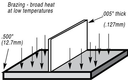
burn through, or at least warp, the thin section. The broader heat and lower temperature of brazing allows you to join the sections without warpage or metal distortion.
