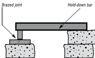
If you have a number of assemblies to braze and their configuration is too complex for self-support or clamping, it may be a good idea to use a brazing support fixture.
