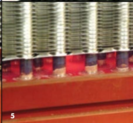
1. Handy One® flux cored brazing alloys are ideal for products such as heat exchangers because they simplify the brazing process and provide stronger, better quality joints.
