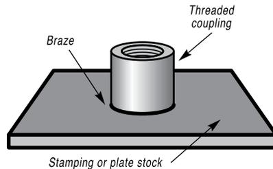
plate is a stamping and the coupling a screw machine part. Weight is down to the bone, too, because the thickness is only where it's needed, in the threaded coupling. Material can be matched to function. And the assembly will undoubtedly be stronger than the casting.
