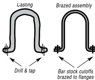
as well as the casting. And it's a lot cheaper to make, because you're putting the thickness only where you really need it—in the flange and not the shell. You save weight, materials and labor.
