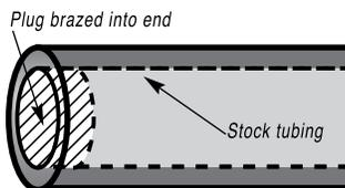
The assembly is a lot less expensive to make than the machined part—and it works just as well.
