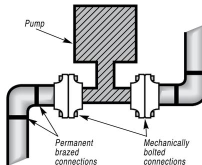
in mind. (For example—a pump connected to a piping assembly.)
