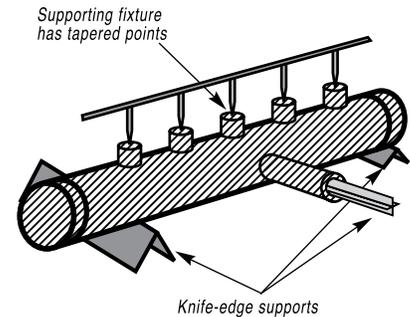
Try to use materials in your fixture that are poor heat conductors, such as stainless steel, Inconel or ceramics. Since these are poor conductors, they draw the least heat away from the joint. Choose materials with compatible expansion rates so you won't get alterations in assembly alignment during the heating cycle.
