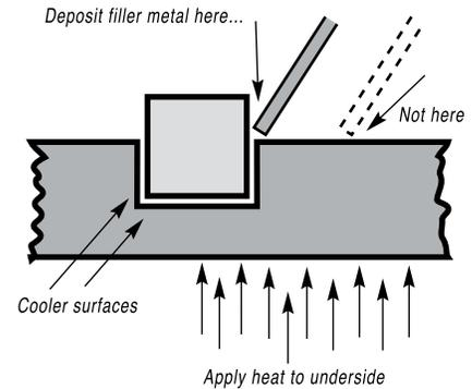
away from the joint, it tends to plate over the hot surfaces rather than flow into the joint. In addition, it's best to heat the side of the assembly *opposite* the point where you're going to feed the filler metal. In the example above, you heat the underside of the larger plate, so that the heat draws the filler metal down fully into the joint. (Always remember—the filler metal tends to flow toward the source of heat.)
