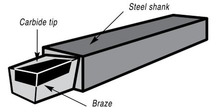
By brazing, you've reduced material cost—obviously. But even more—you're now using metals perfectly suited to their functions. Hard carbide at the cutting edge, and shock-resistant tool steel for the shank.
