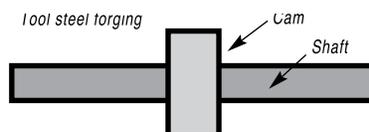
ing, the cam has to be drawn and the shaft ends annealed. How about making the cam and shaft *separately*—and then join them mechanically as an *assembly*?
