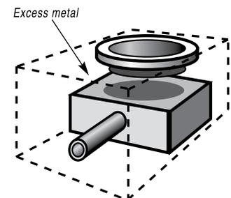
want, and the labor of getting rid of it. There's an easier way. Make the "part" as a brazed assembly, joining together standard tubing and bar stock components:
