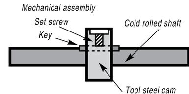
stituting cold rolled for tool steel in the shaft, you're saving on material cost. But machining is still somewhat involved, and a locking device, such as a set screw, is subject to loosening under vibration.
