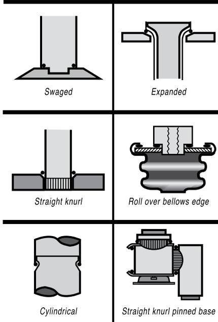
The *simplest* mechanical holding device is the best, since its only function is to hold the parts together while the permanent joint is made by brazing.
