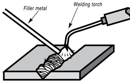
It offers one big plus—strength. Properly made, the welded joint is at least as strong as the metals joined.
