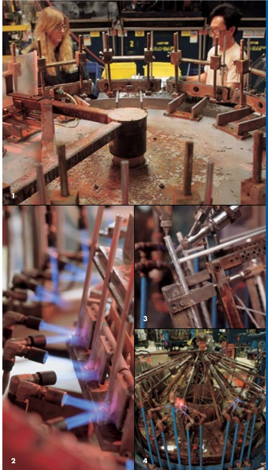
1. Inlet and outlet tubes are brazed at an automated index table.
