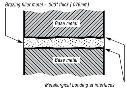
The principle by which the filler metal is drawn through the joint to create this bond is *capillary action*. In a brazing operation, you apply heat broadly to the base metals. The filler metal is then brought into contact with the heated parts. It is melted instantly by the heat in the base metals and drawn by capillary action completely through the joint.
