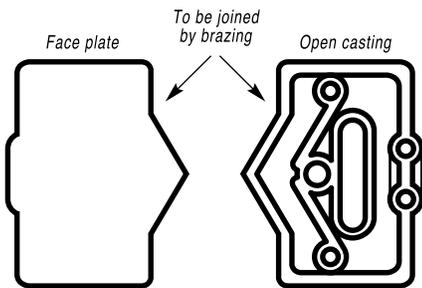
the complex cored casting with a simple open casting—and a metal stamping. Machining is easier, and brazing's capillary action assures you of a leak-tight bond.
