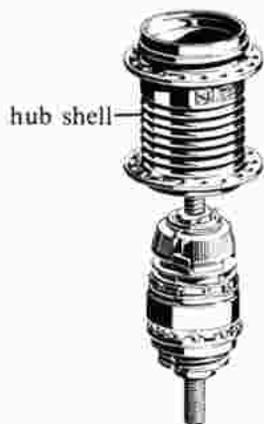
Position hub shell long end up and lower over assembly until it seats.
