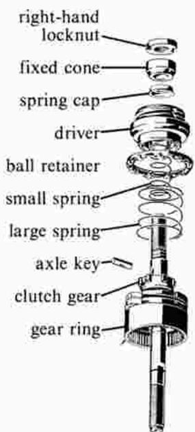
Position axle assembly vertically with right (hollow) end up. Slip gear-ring/clutch-gear assembly over axle with gear ring facing down.
