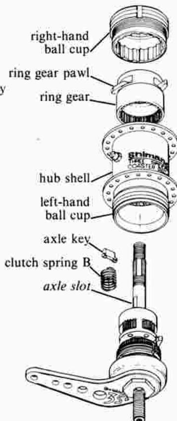
Invert assembly. Install light gauge clutch spring (B). Install axle key *notch down* in axle slot. Slip hub shell over assembly with left-hand ball cup seating against balls in ball retainer. Rotate ring gear pawls into operating position (full clockwise, viewed from above), press in and slip ring gear over axle into hub shell. Thread in right-hand ball cup. Tighten with ball-cup tool.
