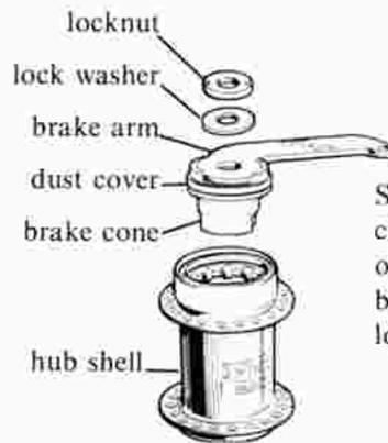
Slip hub shell over assembly. Rotate counter-clockwise until shell race seats on large retainer. Install brake cone, brake arm (brand name facing out) and locknut. Adjust bearing.
