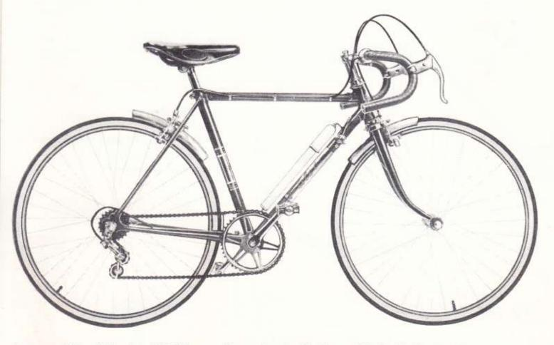
Frame: 18". Wheels: 24" Clement Tyres fitted. Brakes: Side Pull, Hooded Lever.
