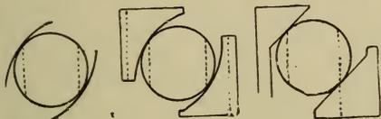
BALL CONTACT IN "TWO-POINT" BEARING.
