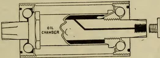
STEARNS SELF-OILING CRANK-HANGER MECHANISM.
