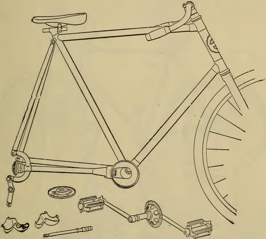
MECHANISM AND FRAME OF COLUMBIA CHAINLESS.
