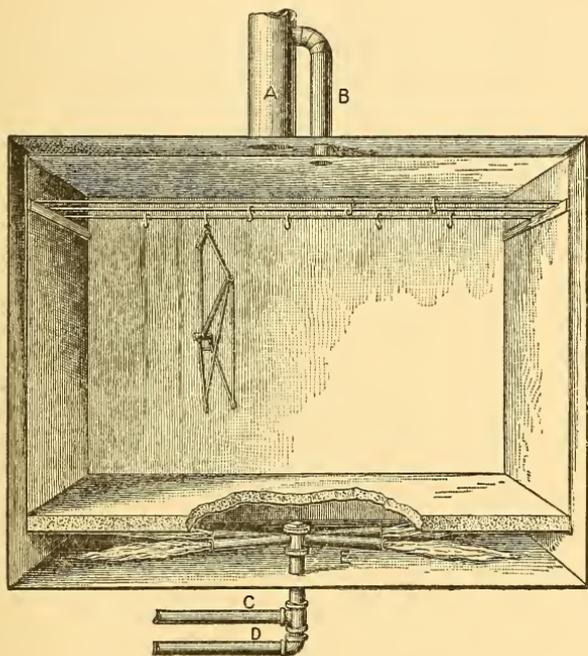
*Fig. 6.—Enameling Oven Heated from Outside.*
