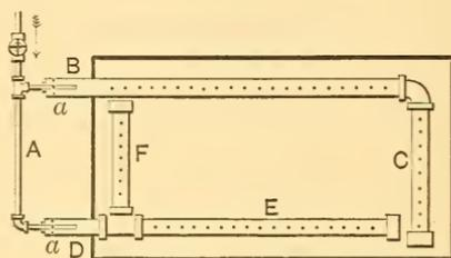
Fig. 5.—Plan of Multiple Bunsen Burner in Fig. 4.
