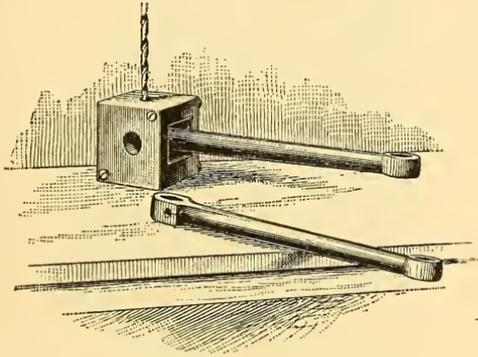
*Fig. 14.—Boring Crank.*
