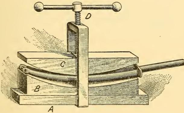
Fig. 4.—Bending Forks.
