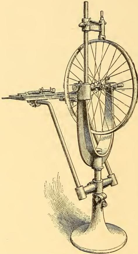
*Fig. 7.—Jack for Holding a Wheel for Truing.*
