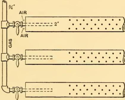
*Fig. 3.—Plan of Multiple Bunsen Burner in Fig 2.*
