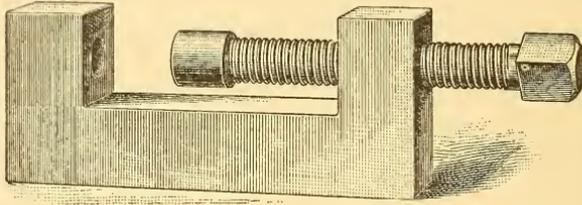
*Fig. 3.—Dog for Removing Keys.*
