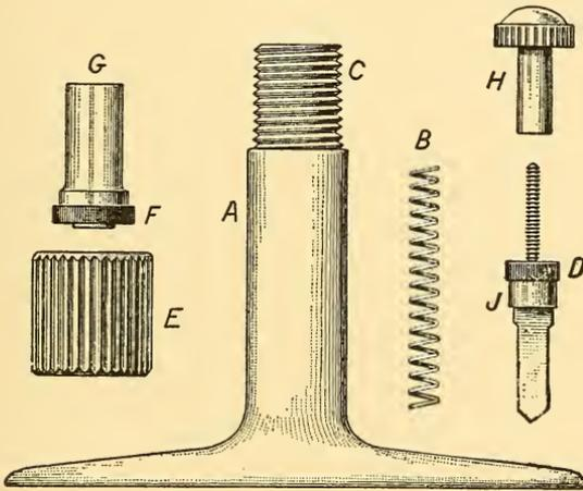
*Fig 4.—Repairing the Valve Proper.*
