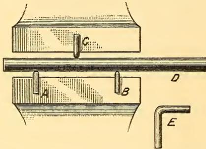
Fig. 18.—Straightening Shafts or Bars in the Vise.
