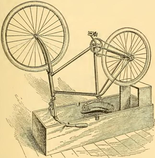
*Fig. 2.—Stand for Holding Bicycle in Inverted Position.*
