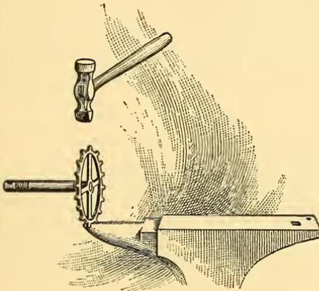
*Fig. 19.—Removing a Screwed on Sprocket.*
