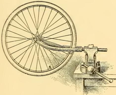
*Fig. 3.—Truing Front Wheel Held in its Fork.*
