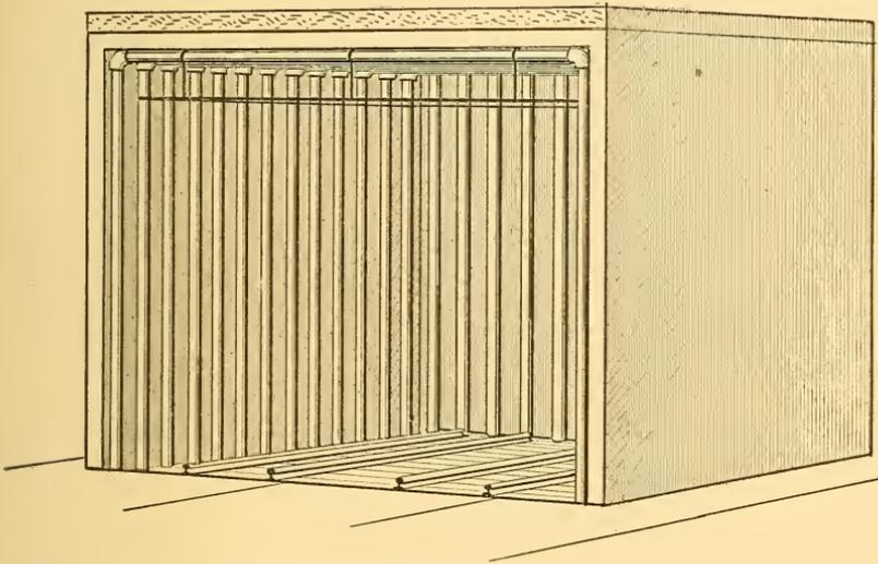
*Fig. 10.—Steam Heated Enameling Oven.*
