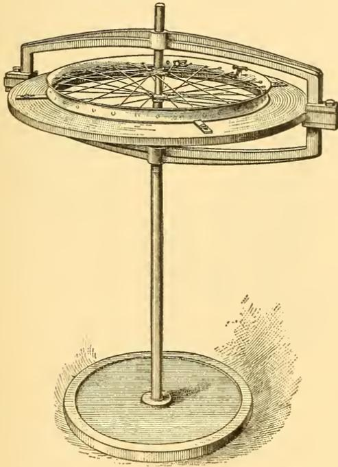
Fig. 11.—Stand with Flat Cast Iron Base.
